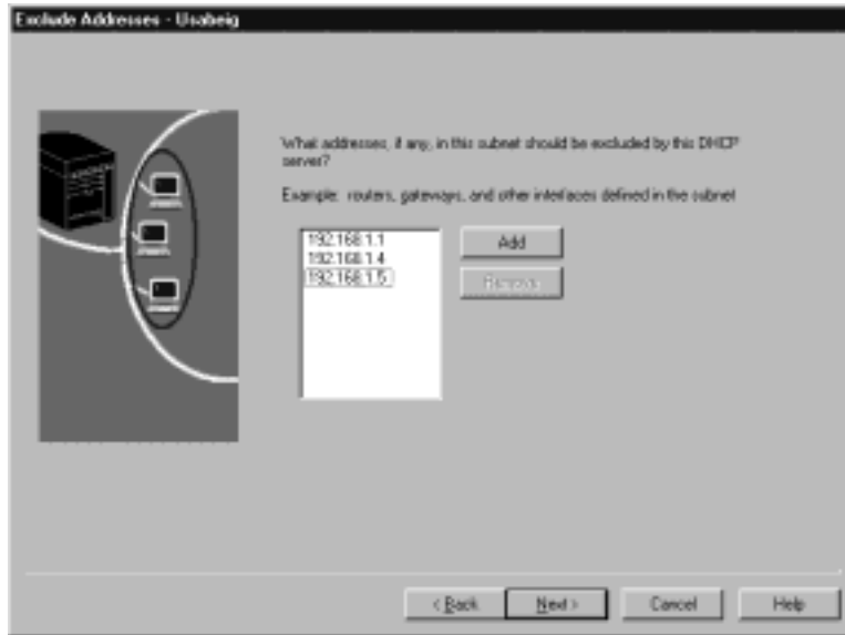
Figure 22. Exclude Addresses. In the Figure 5 on page 7, subnet 9.5.67.0 would exclude the router, server, and the domain name server.
