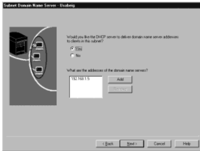
Figure 22. Domain Name Server. Sample configuration for Figure 5 on page 7.
