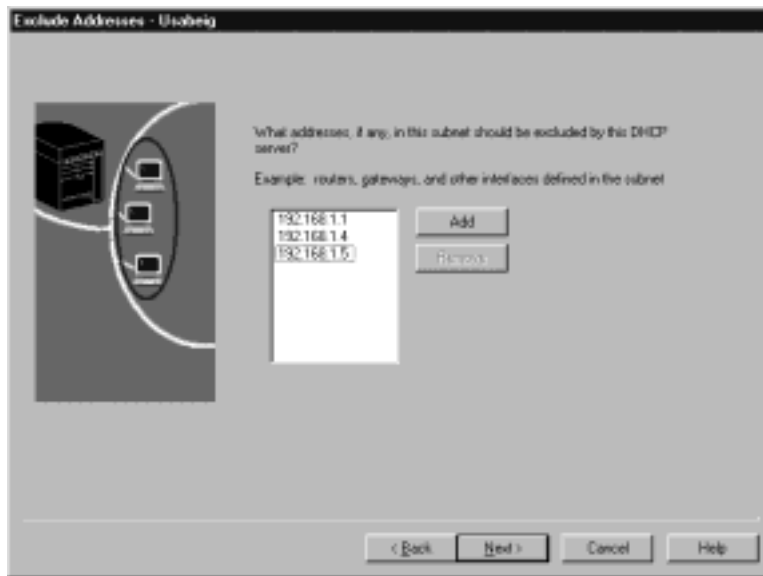
Figure 21. Exclude Addresses. In the Figure 5 on page 7, subnet 9.5.67.0 would exclude the router, server, and the domain name server.
